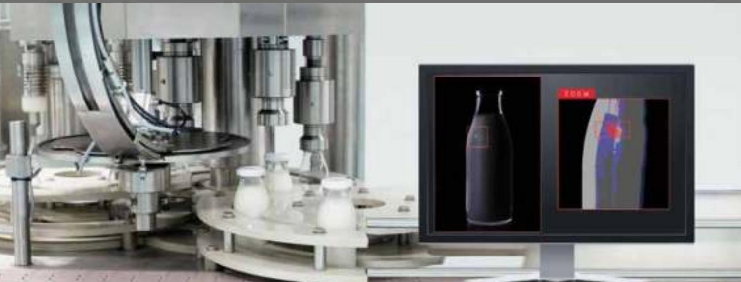
**D-TEKBLUE** is a FDA approved blue PTFE detectable using optical scanner, metal detection equipment or X-ray equipment, whatever the type of food has been processed. This ensures that each fragment can be identified rapidly avoiding critical food contamination.
