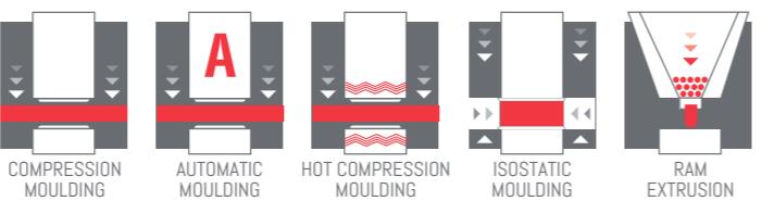
Because of its high viscosity above the melting point, PTFE cannot be processed by means of transformation processes which are standard for the majority of thermoplastics. Specific processing method similar to those used in powder metallurgy had to be developed.
