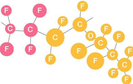
Derived from standard PTFE, modified PTFE is a copolymer of tetrafluoroethylene and a small quantity of a perfluorinated modifier (perfluoropropyl vinyl ether, PPVE). The modifier content is less than 1%.
