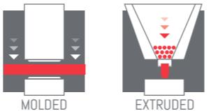
An extensive range of sizes are available to satisfy customers' requirements for **both molded and extruded products**. In addition to virgin PTFE tubes and rods, standard or special compound products are also available.
